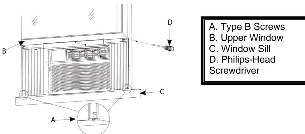
3. Install the window fixing bracket:
