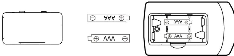
1. Remove the cover on the back of the remote control.
