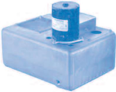
Hartell's AL-2 series pumps are designed to handle the high volume of water produced during the flushing cycle. The AL-2 comes with a 2 gallon cast aluminum reservoir, 6 foot cord and plug, 1 3/8" inlet and 3/8" NPT Female outlet. Maximum water temperature 150° F.
