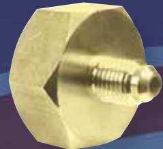
92836 Refrigerant Drum Adaptor 3/4" NPS Cylinder x 1/4" M.F.
