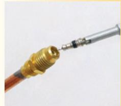
Valve Core Pick Extractor Removes broken valve core
