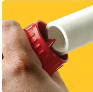
Use inside/outside Deburring Tool [Uniweld Part# 70079] to remove burrs from pipe.
