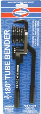
A compact and durable tool with multiple bending channels that is capable of bending 1/4", 5/16" and 3/8" O.D. soft copper, aluminum and soft stainless steel tubing. Calibrated markings show angle of bend for accurate left hand, right hand and offset bends up to 180°. 1" bend radius.
