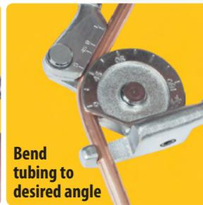
Bend tubing to desired angle
