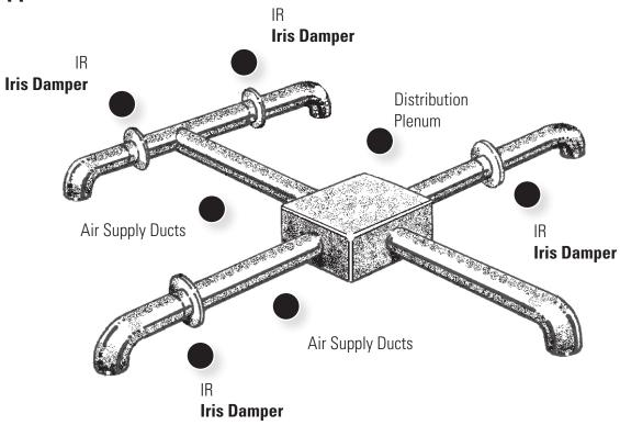
Typical multi-duct installation where Iris Dampers are used to balance the system.
