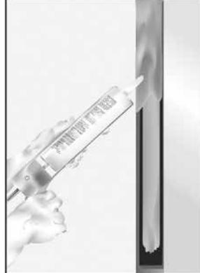
3. Gun, trowel, or pump approved sealants to minimum 1/4" depth on both sides of wall or top of floor over the backer rod.
