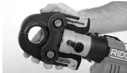
Figure 4 – Sliding The Attachment Out of the Tool
