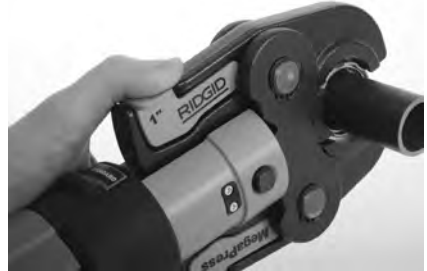
Figure 8 – Opening the MegaPress Jaw set and Placing Around Fitting
