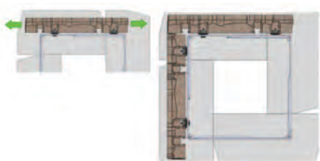
Take another stone and repeat the same process. Make sure you have a corner stone to finish the corner. Once installed, slide the stone along the horizontal axis to adjust the corner.
