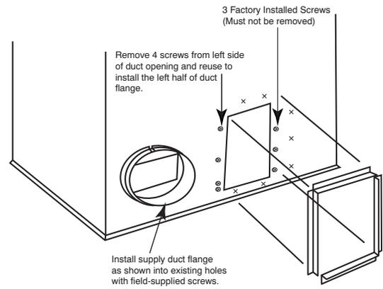
X = Factory dimples for duct flange attachment.
