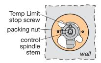
Figure 3 Valve adjustments
