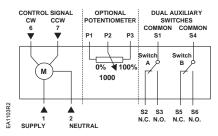
0 to 10 Vdc, GCA16x, 24 Vac/dc; 2 to 10 Vdc, GCA15x, 24 Vac/dc:
