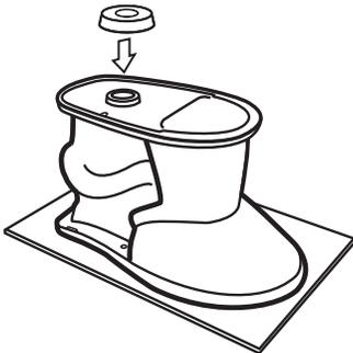
Remove the toilet from the box and set the toilet upside down on a soft surface. (You may use the box for this purpose.) Set the wax ring firmly in place around the outlet of the toilet.
