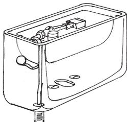
Install the toilet tank which has been factory assembled. The gasket seal is between the bowl and the bottom of the tank and is ready to set in place. Place the tank on the toilet bowl. Slide the tank toward the front or back of the bowl until the desired gap, normally 1/2 to 1 inch, is obtained between the tank and the wall. Secure the tank in place with the two (2) metal washers and two (2) wing nuts provided. **DO NOT OVERTIGHTEN.**
