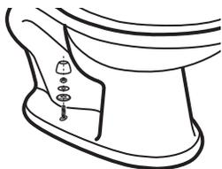
Install the plastic washer (be sure that the side marked “top” is facing up), round metal washer, and full hex nut. **DO NOT OVERTIGHTEN.** Cut off any excess bolt length and snap the bolt cap in place. Run a bead of caulk around the base of the toilet for a finished look and to meet plumbing codes.
