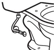
Connect the water supply to the toilet fill valve and hand tighten. Carefully connect the water supply to the shut-off valve.
