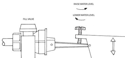
Open the shut-off valve slowly and check for leaks. Fill the EcoLogic® dump bucket to the water line. Adjust the level if necessary by turning the black screw on top of the float. Turn the screw to the right to lower the water level or to the left to raise the water level.
