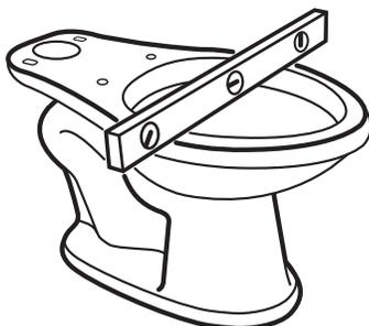
Make sure that the toilet bowl is level. If the toilet tilts or is rocking, insert shims under the base.
