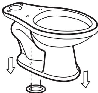
Carefully lower the toilet bowl onto the floor flange while aligning the "T" bolts through the two holes in the toilet bowl foot.
