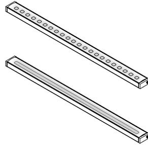
A typical LED fixture creates LED hot spots.
