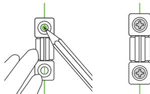
b. Mark holes. Use min one clip for every foot of channel. Fasten with applicable screws w/ screwdriver or drill.
