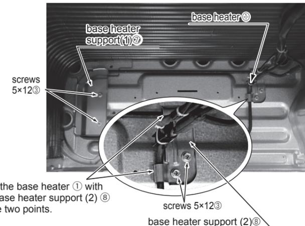
Hold the base heater ① with the base heater support (2) ⑧ at the two points.
