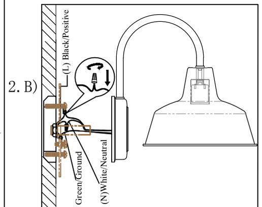
Step.2 Wire fixture to wires in outlet box. Black wire is positive, white is neutral, bare wire is ground.
