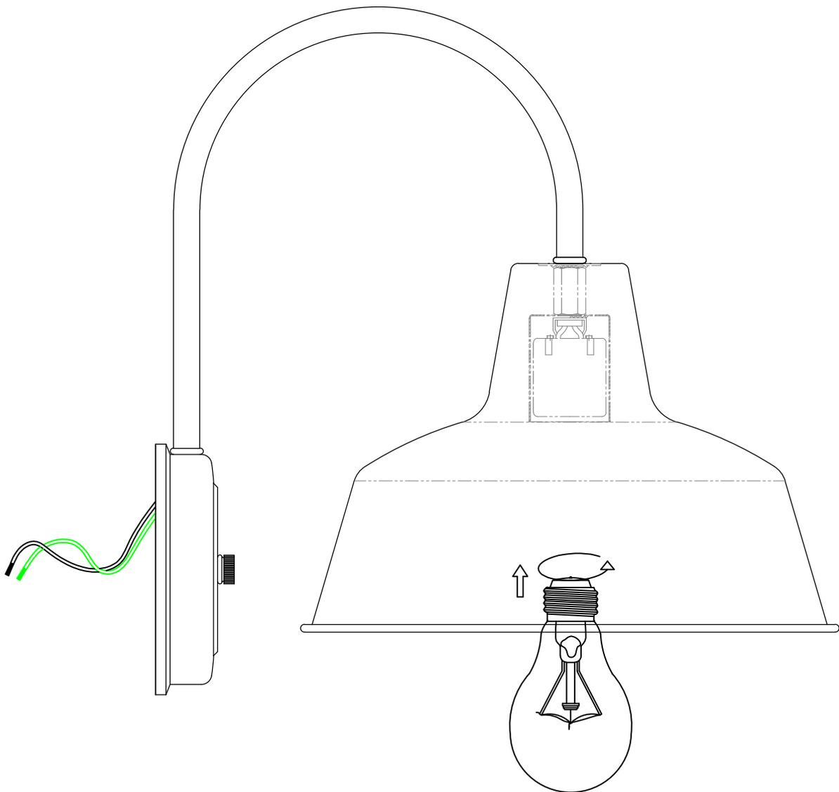
**WARNING:** To prevent water intrusion, caulk around back-plate where fixture meets the wall using outdoor silicone sealant. Leave a small gap at the bottom to allow moisture to exit.
