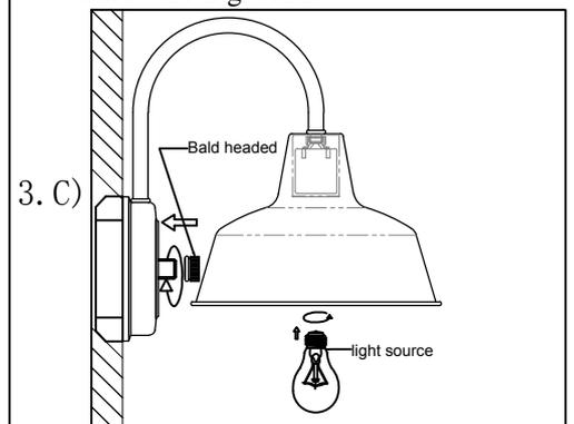
Step.3 Put the connected line into the electric box and fasten the light body with the decorative nut.
