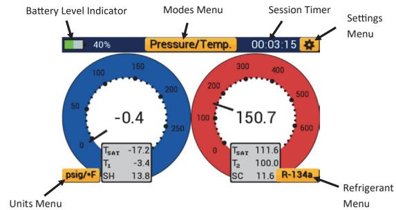
Pressure/Temperature Mode displays system pressure, temperature, saturation temperature, system superheat and subcooling. Settings can be accessed by tapping the settings icon in the upper right corner. The modes menu can be accessed by tapping the button labeled with the name of the current mode at the top of the screen. The units and refrigeration menus can be quickly accessed by tapping the buttons in the lower left and right corners respectively.
