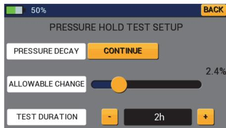
The Pressure Hold mode displays the change in pressure of the system during a standing pressure test. Allowable change is the percentage of the current system pressure the system is allowed to drop before the pressure test is deemed a failure. Set the allowable change percentage by adjusting the slider bar. Adjust the duration of the pressure Decay test by tapping the "+" and "-" buttons. Tap the Continue button next to Pressure Decay to begin the pressure hold test.
