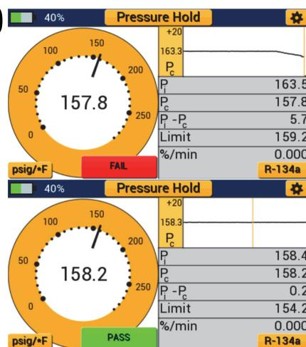
Tap Set Pi to set the initial pressure and begin monitoring for a drop in system pressure. The device will display a Fail or Pass message depending if the system Fails or Passes the pressure Decay respectively.
