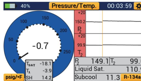
While in Pressure/Temperature mode, tapping the center of either gauge will convert the gauge into a graph. Tap the center of the graph to convert the graph back to a gauge.
