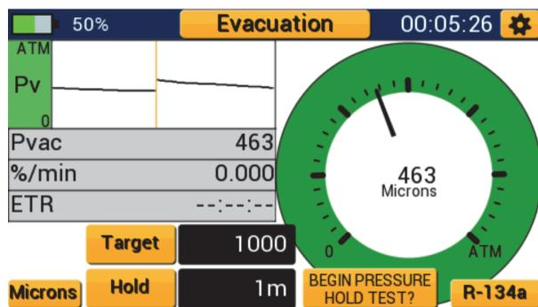
Once the Vacuum Hold timer has depleted, the user is prompted to start a pressure hold test. Tap the button to advance to the pressure hold setup screen.
