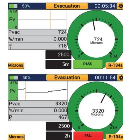
The Pressure Rise test will monitor the current vacuum pressure and the percent change in pressure. The device will prompt the user with a Pass or Fail message depending if the system passes or fails the test respectively.
