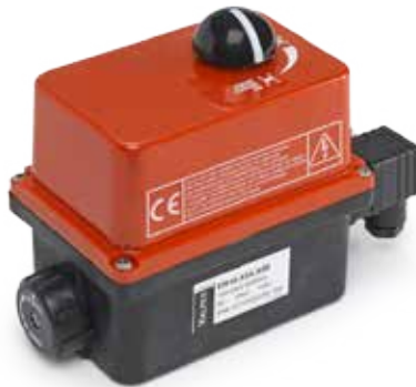
Electric actuator has been designed to control valve with 90 deg rotation 15W, IP66. Option 1: 90-240V, 50/60HZ, 90-350V DC, Option 2: 15-30V, 50/60HZ, 12-48V DC
