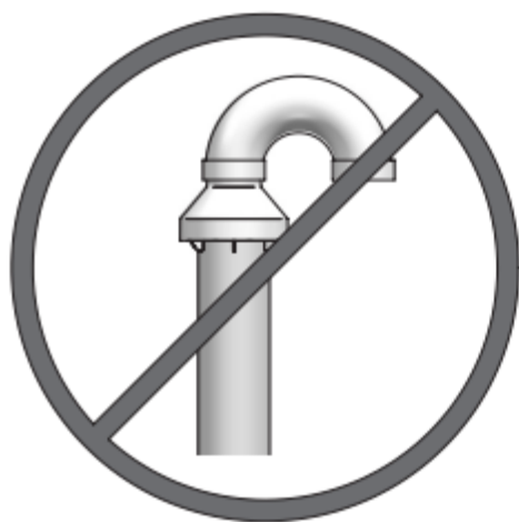
Figure 5-5 Do Not Install U-Bend to Rain Cap
