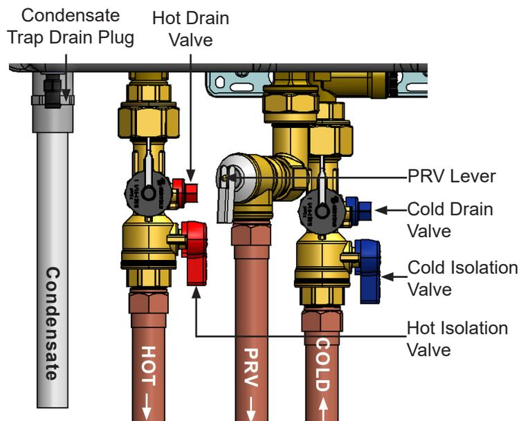
Figure 77: Piping Diagram
