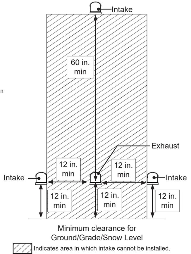
Figure 33: Horizontal Vent and Combustion Air Piping
