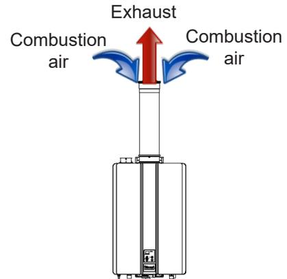
Figure 23: Concentric Pipe
