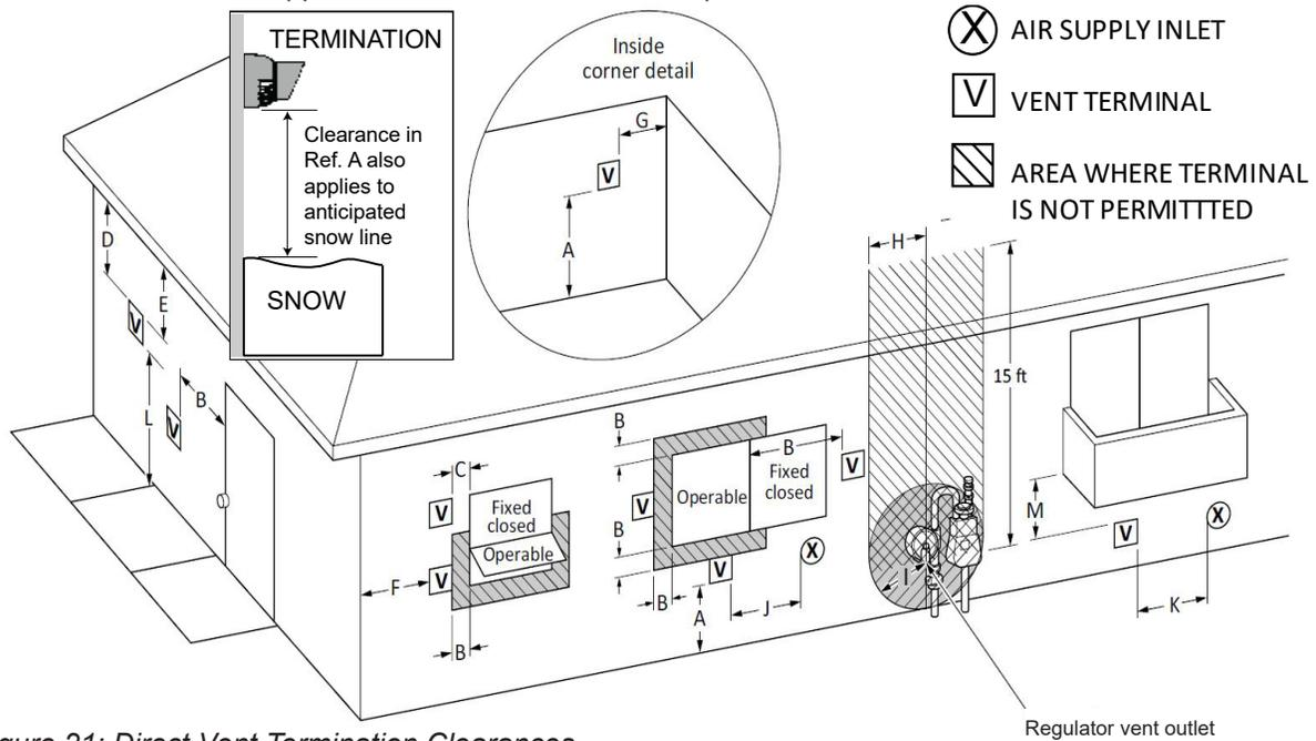
Figure 21: Direct Vent Termination Clearances
