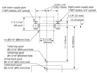
X", # = At least 5" clearance from sensor to tip of toilet seat up position or to top of grab bar is required to avoid false detection.
