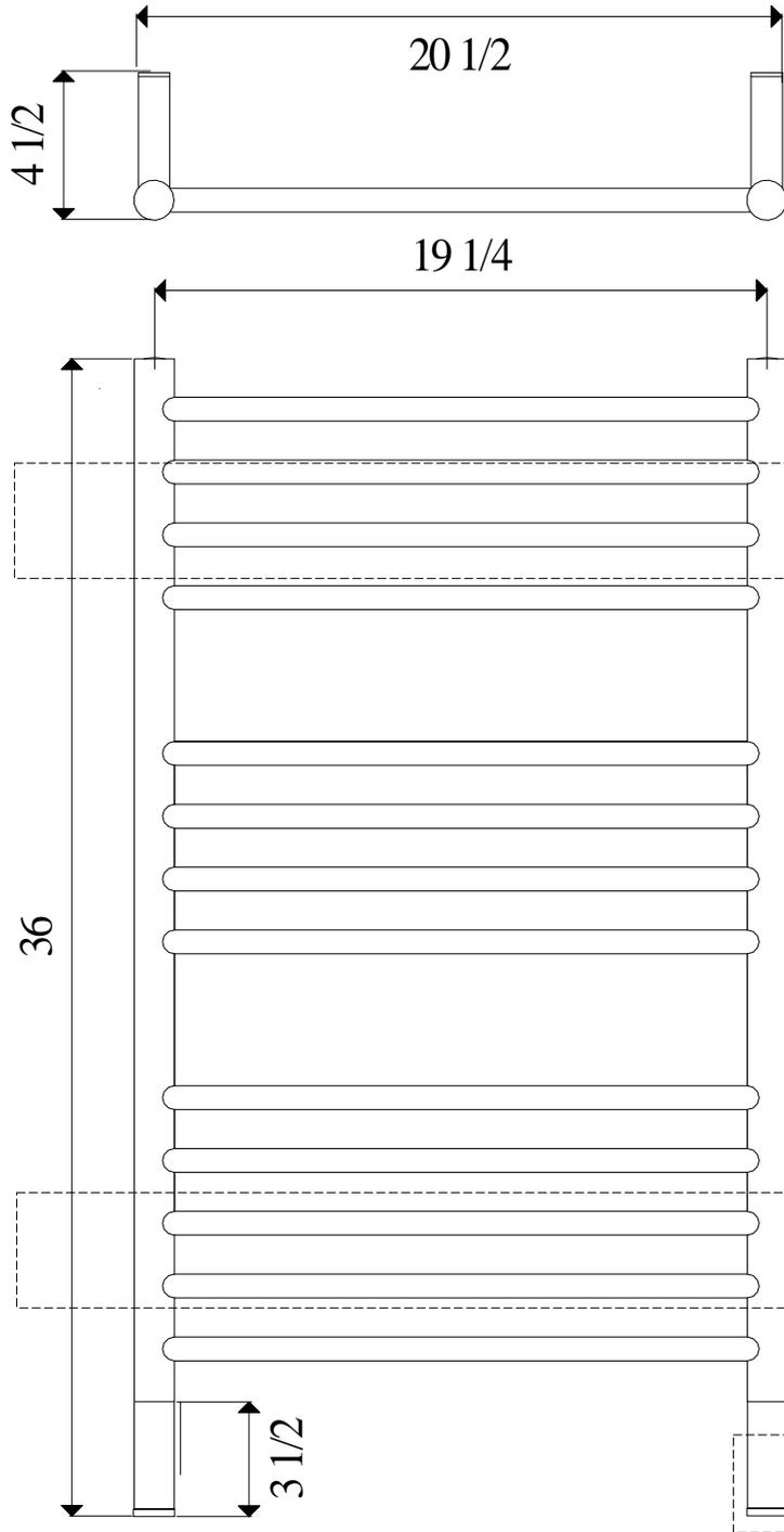
For construction with wall studs on 16 in. centers, the header is located between the studs for the right side mounting. For construction with wall studs on centers greater than 19-1/2 in. provide secure header as shown.
