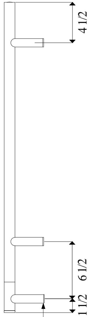
Wire cover tube fits into centre of cover plate which fits over single gang box
