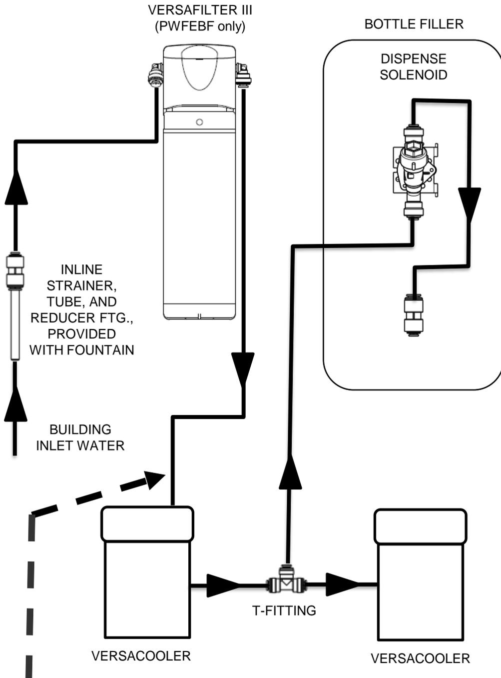
**IMPORTANT:** Flush filters before connecting water line to VersaCooler. PWFEFB only.
