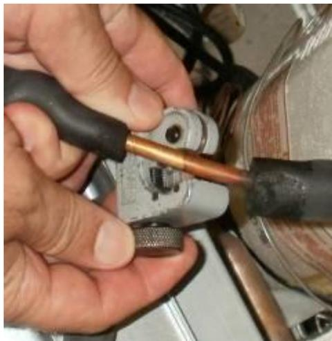
4. Install TEE fitting by connecting the copper tubing to each end. Then install the 32" piece of plastic tubing to the TEE branch.
