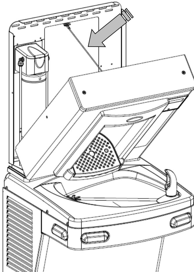
3. Before the Bottle Filler cabinet is set into place, feed the terminals on the power supply power cord and the long green ground wire through the bushing on the cooler top.
