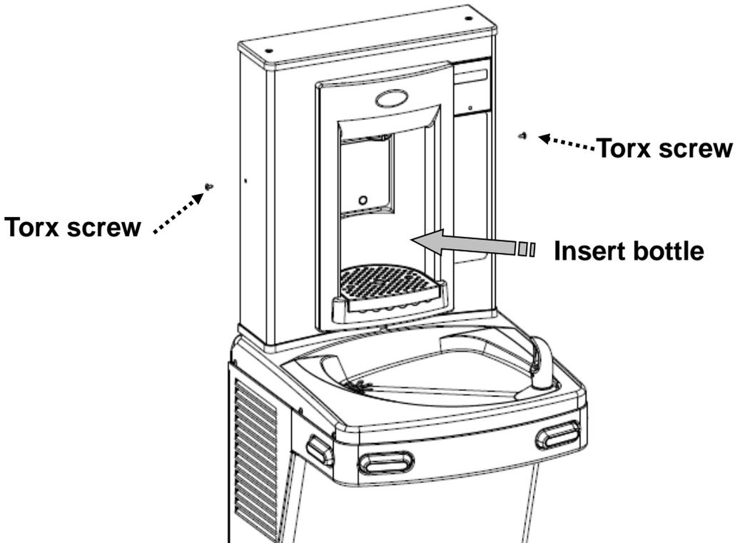
7. Attach Bottle Filler assembly to the frame using two (2) torx screws. If you are going to change the electronics default settings, remove the Top Cap and two (2) torx screws.
