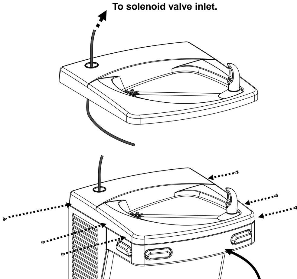
**TIP:** For the P8AM, it is easier to connect the outlet tube to the bubbler if the front nose is removed.
