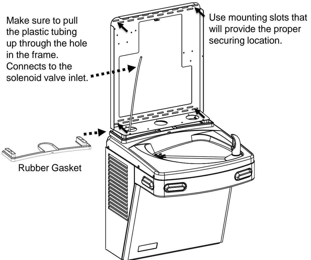
3. Secure frame to the wall with fasteners (not provided). Pull plastic tubing up through the hole in the frame.
