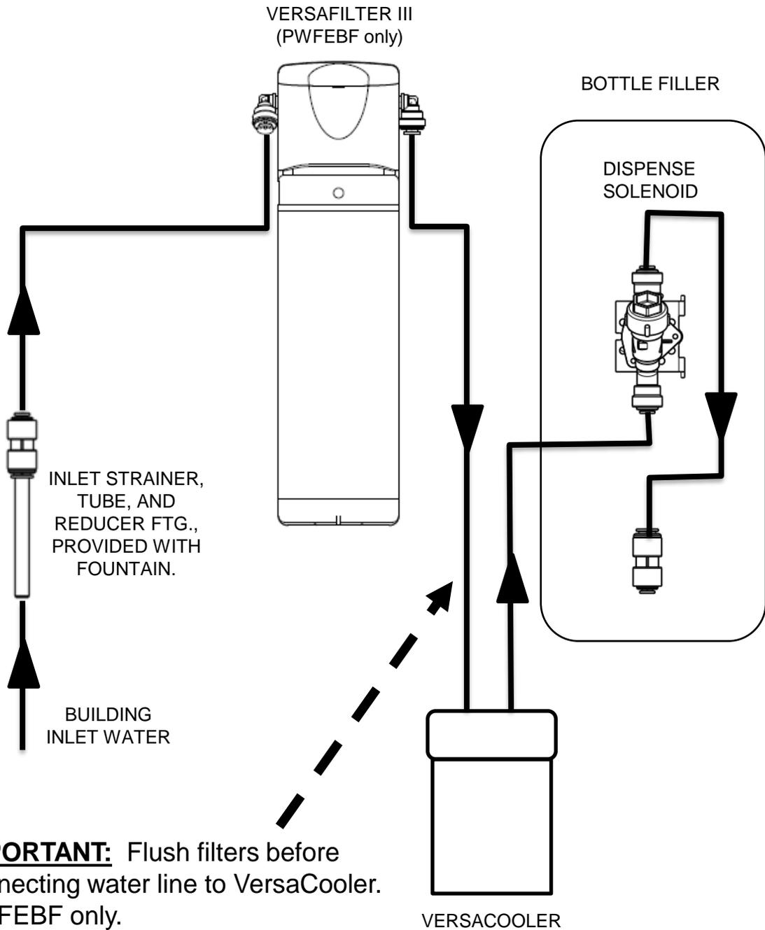
**IMPORTANT:** Flush filters before connecting water line to VersaCooler. PWFEFB only.
