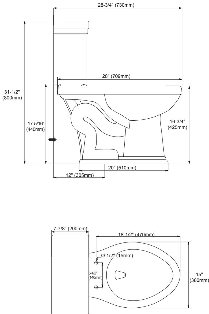
Note: All dimensions and specifications are nominal and may vary: Dimensions of 8" and greater have a tolerances of +3%. Dimensions less than 8" have a tolerances of +5%.
