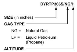
H = High Altitude Model, 4000 ft.(1219 m) and up No character = Equipped for low altitude operation
