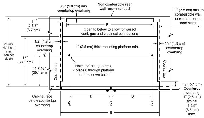
**NOTE:** Gas and electrical connections may only be routed through the bottom of the rangetop when installed with a downdraft vent.
