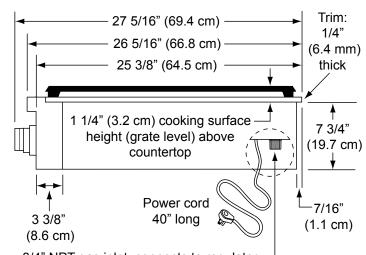
3/4" NPT gas inlet, connects to regulator – from bottom or rear of unit, end is recessed 2" (5.1 cm) from chassis bottom
