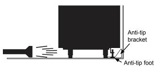
6. With a level ensure the range tnot tilt front to back or side to side. (Adjust the legs as needed.)
