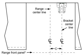
4. Place the bracket against the wall in the mounting location. Using a 1/8" bit, drill four 1-5/8" deep pilot holes perpendicular to the screw-seating surfaces shown below. Attach the bracket to the wall as shown with the included #12 x 1-3/4 screws.
