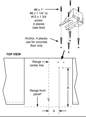
Determine the screw size required. The minimum full thread depth (portion of screw threaded into wood/slab) for wood is 3/8" (1 cm) and 5/8" (1.6 cm) for concrete. See SCREW SIZE TABLE to select the correct screw size.
