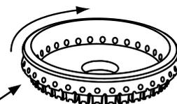
**STEP 1:** Put burner ring on top of head.
