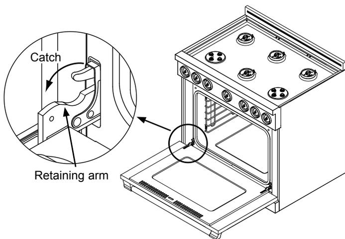
3. Lift the oven door to about a 15° angle from the vertical position.
