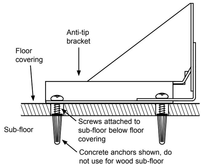
Four (4) plastic anchors are provided along with three sizes (4 each) of #8 or #12 Phillips head screws for attaching the anti-tip bracket to the floor. Use both the anchors and four (4) of the screws when attaching the bracket to a concrete sub-floor. Do not use the provided anchors when attaching to a wood sub-floor.
