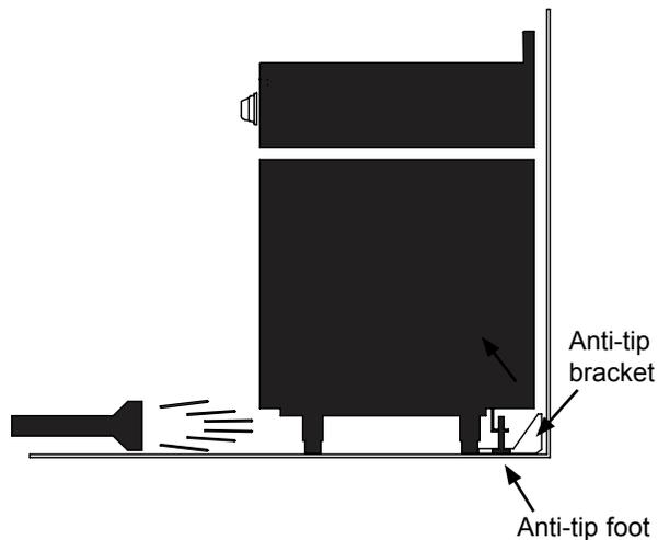
5. Use a level to make sure that the range does not tilt front to back or side to side. Re-adjust the legs to level and change the height if necessary.
