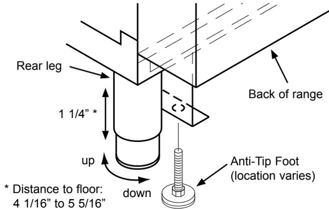
4. Carefully slide the range into position into the cutout. The anti-tip foot should engage the anti-tip bracket. Using a flashlight look underneath the range and verify that the bracket covers the anti-tip foot.
