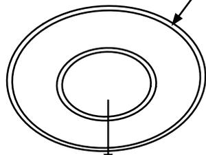
**STEP 2:** Install burner ring. Line up ring tabs with head slots.
