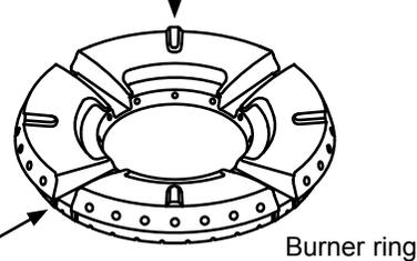
**STEP 1:** Install burner head. Put locating tab in keyed hole.
