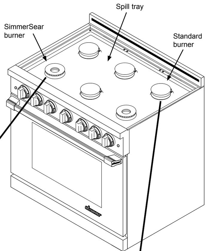
**STEP 3:** Install burner cap. Ridge on cap must surround top of ring.
