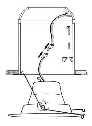
Insert the torsion springs into the fixture housing brackets. Gently push the product up and torsion springs so they begin to expand and lift the product in place.
