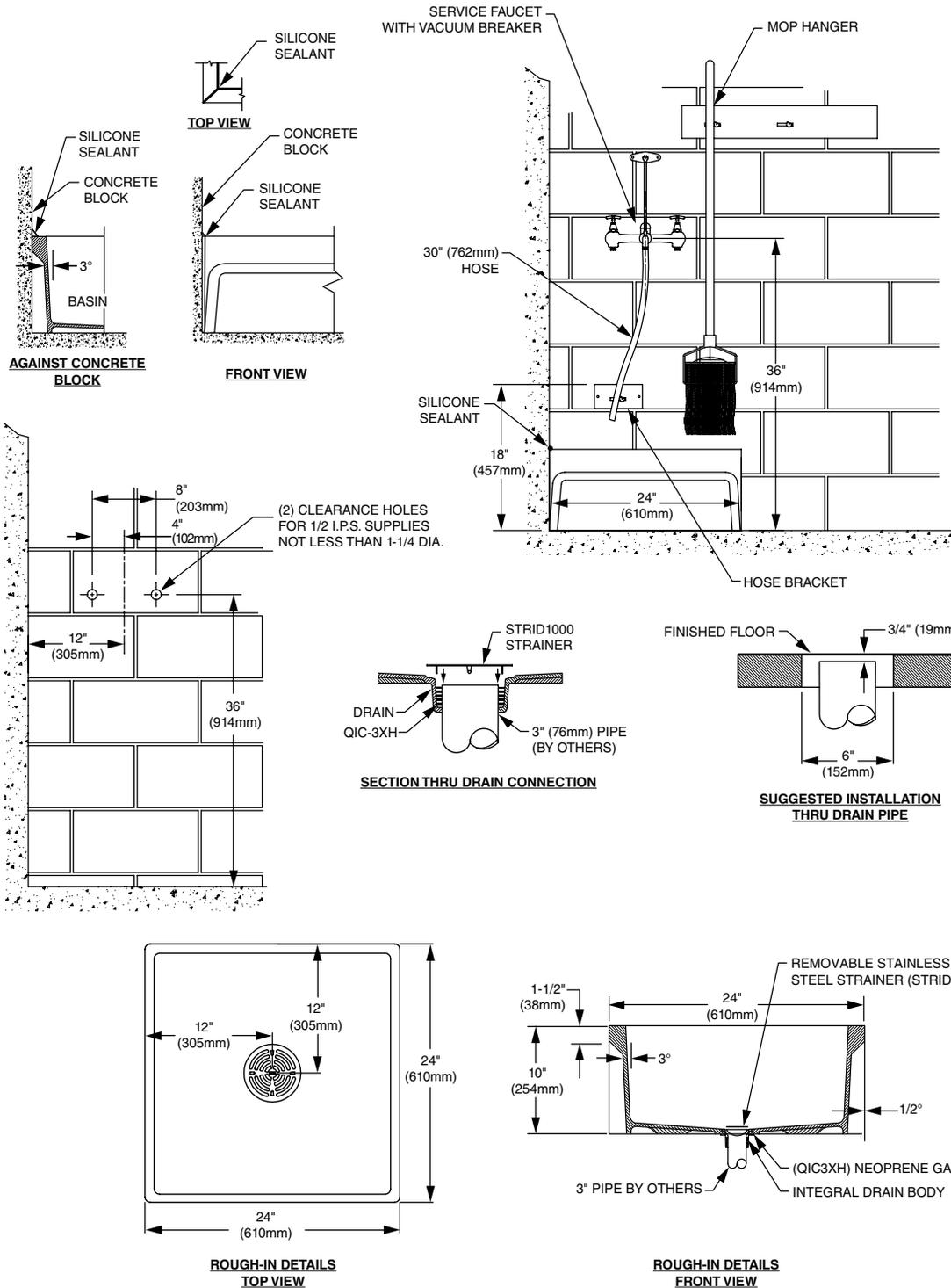
**Installation Note :** QIC32 Quick Drain Connector for 2" pipe or QIC3SN Quick Drain Connector for cast iron soil pipe must be ordered separately.
