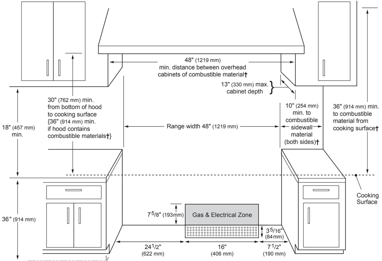
† as defined in the "National Fuel Gas Code" (ANSI Z223.1, Current Edition). Clearances from non-combustible materials are not part of the ANSI Z21.1 scope and are not certified by CSA. Clearances of less than 12" (305 mm) must be approved by the local codes and/or by the local authority having jurisdiction.
