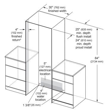
\*A minimum 4" (102 mm) finished return that matches the cabinet exterior is recommended on all sides and the top of the cutout opening. The shaded area will be visible after installation.
