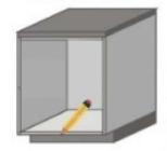
Mark drain hole position on cabinet, drill 3/8" hole for drain cone. Cut tip off drain cone.
