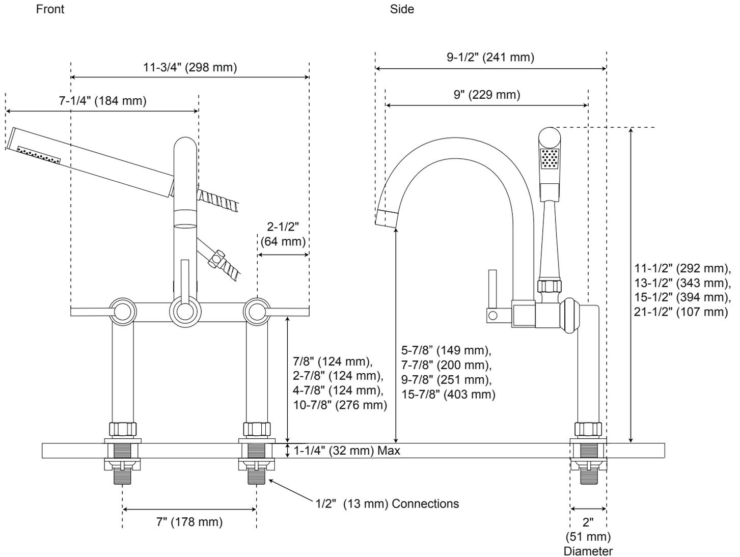
Faucet spout extends below deck when installed with 2" couplers.
