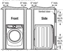
\*Installation with steam dryer requires additional 3/4" hose clearance.
