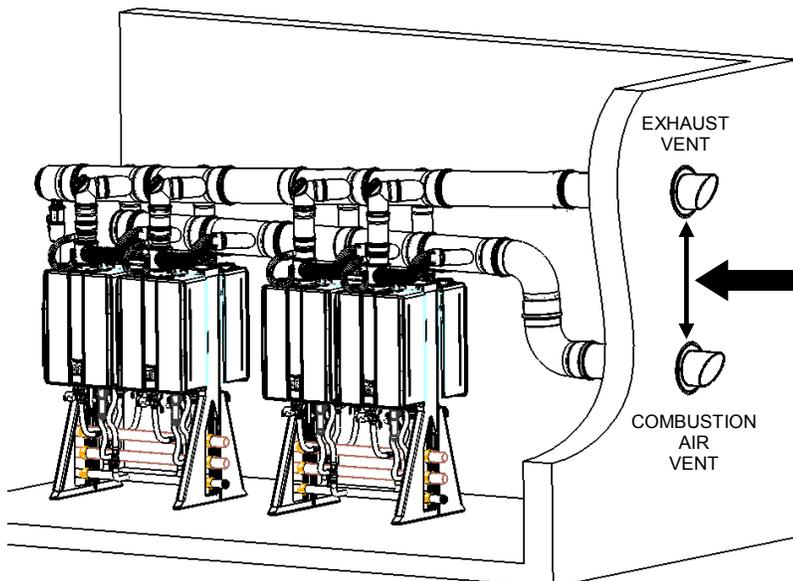
**NOTE:** During colder weather when the exhaust temperature is much hotter than the outside air, the exhaust fumes condense producing water vapor. As a result a plume of water vapor may be seen leaving the exhaust.
