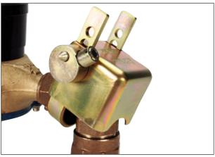
**STEP 5.** Install the Mitey Lock body over the locking pin and secure it with a short length barrel lock. The installation is complete and the valve is secured.
