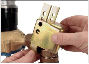
**STEP 3.** Place the shroud over the valve while guiding both legs of the strap through the slots in the shroud. Align the adjustment holes in the strap with either upper or lower holes in shroud. Try to achieve the tightest fit possible.
