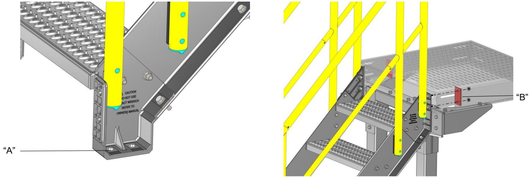
With the stair assembly fully assembled (in this configuration, tower supported) no stair to platform bracket is required), properly locate the stair unit on the pad layout anchor bolts "A".
