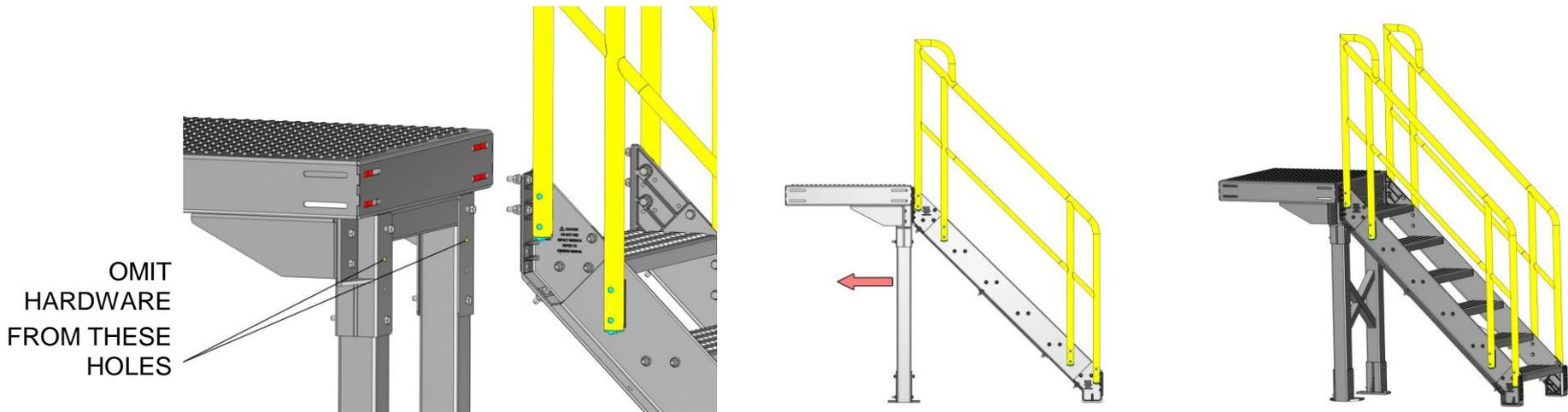
When tower and stairs are both used at the end of a platform, omit indicated hardware from tower assembly. These bolts will interfere with top step of stair unit.
