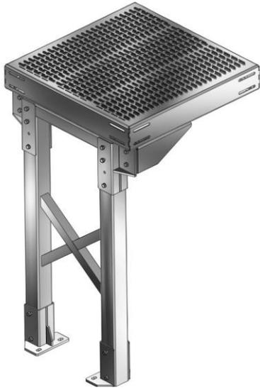
Flush bolting arrangement used when supporting one platform.
