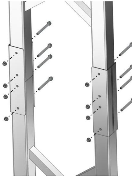
STEP 2: At each stacked section joint, attach brackets and add hardware as shown and tighten hardware.
