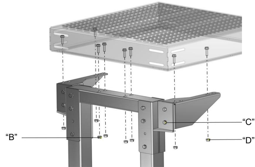
When a platform is being supported by a tower support at the stair location, **the tower should be first located on the anchor bolts and secured in the final assembly location.**
