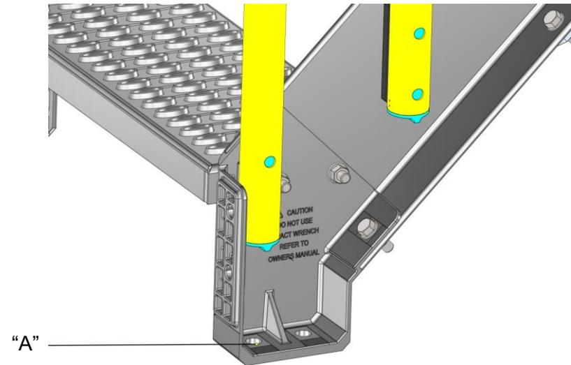
With the stair assembly fully assembled, properly locate the stair unit on the pad layout anchor bolts "A".
