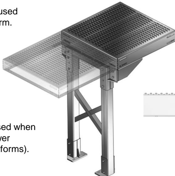
Split bolting arrangement used when supporting two platform (tower located at joint between platforms).
