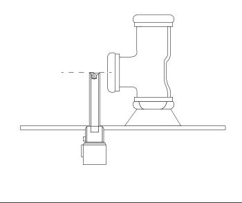
3. Carefully set the tub in position. If the tub has leveling feet, adjust as necessary until level and apply a generous bead of silicone under each foot. If your tub does not have leveling feet, shims can be used for leveling if your floor is not flat.
