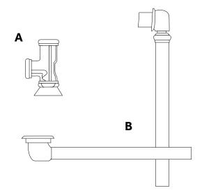
7. Measure and mark each pipe so that the end of the pipe reaches at least a little bit over halfway into the overflow tee.
