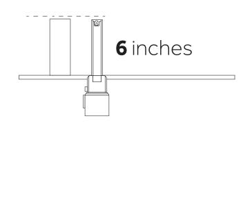
3. When the floor is finished, measure and cut the drain pipe to the appropriate length for the type of drain that is being used.
