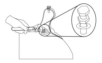
4. Small gaps between the feet and tub are normal, however, plastic or wood shims can be inserted between the tub and the foot's mounting hardware to accommodate. Adjust the shim and locknut until you reach the desired look.
