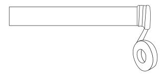
10. Apply 100% neutral cure silicone sealant to the underside of the drain flange and thread it through the tub and into the drain pipe. Apply thread sealant or plumber's tape to the threaded connection to ensure a water-tight seal. Tighten by hand. Wipe away any excess sealant using a damp cloth.
