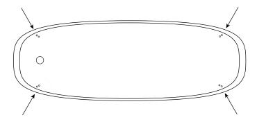
3. Use the provided hardware to attach each foot to the tub. Thread the lock nut onto each mounting bolt, followed by the metal washer. Tighten each bolt firmly with an adjustable wrench.
