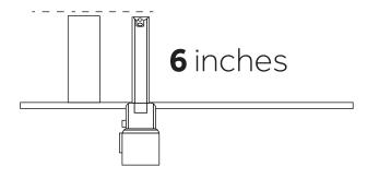
3. When the floor is finished, measure and cut the drain pipe to the appropriate length depending on the type of drain being used, and the distance from the floor to the drain hole.
