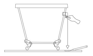
2. Move the tub away from the installation location so that the floor plumbing can be installed. Place the drain pipe at the appropriate height for the waste and overflow piping. To determine this, you will need to temporarily fit your drain pipe into the tub and measure from the floor to the center of the drain pipe.
