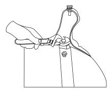
5. Once the feet are in position and adjusted appropriately, tighten the nuts that were used to secure the bar to the bottom of the tub.
