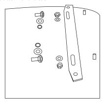
2. Place the provided metal bars over the threaded studs.
