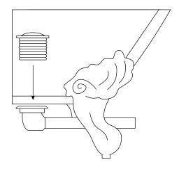
11. Install the overflow assembly with the beveled washer, overflow plate, mounting screw (provided) and any other washers or rubber sealing gaskets included. Apply a bead of silicone sealant to the underside of the flange. If your tub came with a 'Press and Seal' overflow, the pop-up flange will be used in place of the overflow plate and screw.
