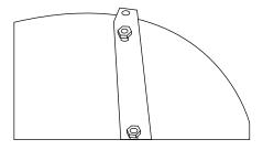
4. Fit the foot to the metal bar and tub. Secure the foot to the end of the bar with the flat washer, locking washer, and bolt.
