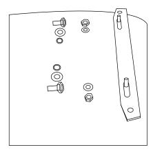
3. Thread a washer and nut onto each stud. Do not fully tighten the nuts; the bar needs to be able to slide back and forth to allow adjustment until the foot is attached.
