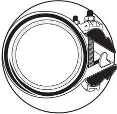
Once the HYMAX Clamp is positioned around the pipe, re-engage the side compression beam over the lug assembly by pushing it downward until it clicks in place TWICE.
