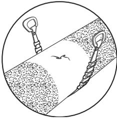
Thoroughly clean and de-scale the pipe surface where the clamp is to be installed. The pipe surface should be free of dirt, corrosion and debris.
