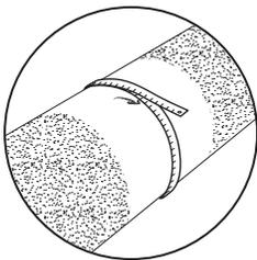
Measure the pipe TWICE using an OD tape. Select the appropriate clamp to fit the outside diameter of the pipe. Unpack it carefully.
