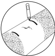
Mark the pipe an even distance from the break or leak according to the length of the HYMAX Clamp.
