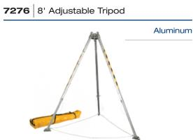
Extruded aluminum 2-stage adjustable legs provide 5' to 8' working height, includes two head-mounted pulleys and two anchoring auxiliary eyebolts, leg-securing safety chain and steel feet with non-slip pads. Offers 55" to 91" internal working height and includes 70" storage bag.
