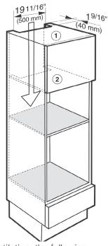
To ensure that the Combi Steam Oven has adequate ventilation, the following cut-outs measuring 19 11/16" x 1 9/16" ( $500 \times 40$  mm) must be made:
