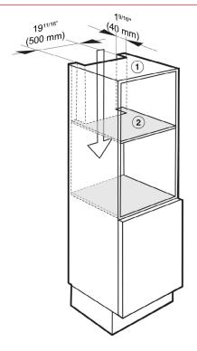
To ensure that the Combi Steam Oven has adequate ventilation, the following cut-outs measuring 19 11/16" x 1 9/16" (500 x 40 mm) must be made:
