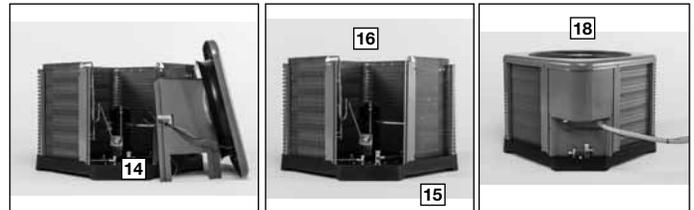
All units utilize strong formed louver panels which provide industry leading coil protection. Louver removal for coil cleaning is accomplished by removing one screw and lifting the panel out of the composite base pan. (17) All RA17 units utilize single row coils (16) making cleaning easy and complete, restoring the performance of the air conditioner back to out of the box performance levels year after year.
