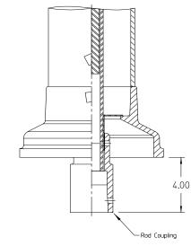
The IP 16 Indicator post does not require disassembly to connect the rad coupling to the gate valve. The IP 16 post rad coupling extends approximately 4 inches below the base, as shown, to allow for an easy connection to the valve wrench nut.
