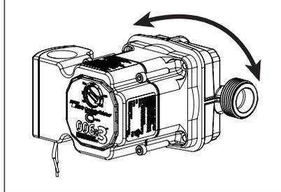
To rotate the pump casing, remove the 4 motor screws using a 5/32" (4 mm) allen wrench. **When rotating pump casing position, DO NOT detach motor housing from the casing.** Damage to the casing O-ring and leakage may result. Simply spin casing to the proper flow direction desired as shown in Figure 4 and Figure 5. Reattach the 4 screws. Be sure motor is positioned correctly and is seated evenly to prevent leakage or damage to O-ring. Tighten motor screws evenly to **25-33** in-lbs torque.
