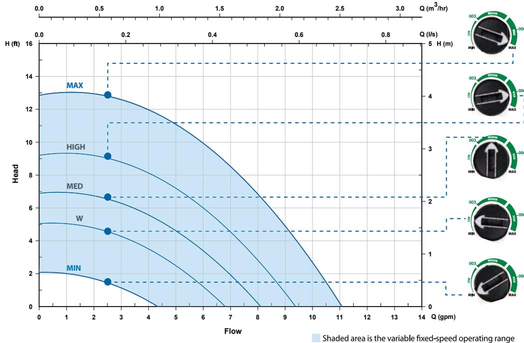
3 fixed speed settings (MIN, MED, HIGH) allows the installer to choose the speed and flow rate to precisely match system requirements. It also has infinitely variable speed settings between MIN/MAX to fine tune flows more precisely. Pre-marked 003/006 settings enable installers to set 006e3 to match standard 003 or 006 performance.
