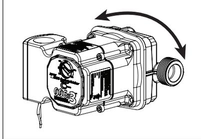
To rotate the pump casing, remove the 4 motor screws using a 5/32" (4 mm) allen wrench. **When rotating pump casing position, DO NOT detach motor housing from the casing.** Damage to the casing O-ring and leakage may result. Simply spin casing to the proper flow direction desired as shown in Figure 4 and Figure 5. Reattach the 4 screws. Be sure motor is positioned correctly and is seated evenly to prevent leakage or damage to O-ring. Tighten motor screws evenly to 25-33 in-lbs torque.
