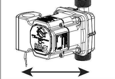
Always install with motor in horizontal orientation. Position electrical junction box at 9 o'clock for best viewing orientation. Pump casing may be rotated to change flow direction. Locate the arrow on the casing body to determine flow direction.
