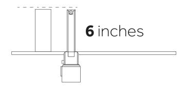
3. Trim the  $1-\frac{1}{2}$ " PVC drain pipe extending from the floor to the appropriate length. This can be determined by attaching the drain to the tub and measuring the distance from the finished floor to the center of the fitting socket.
