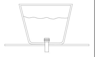
8. Finish your installation by running a bead of neutral cure silicone sealant around the base of the tub where it meets the floor. Wipe away any excess sealant with a damp cloth.
