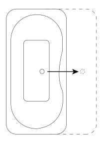
6. Apply 100% neutral cure silicone sealant to the underside of the drain flange and thread it through the tub and into the drain pipe. Apply thread sealant or plumber's tape to the threaded connection to ensure a water-tight seal. Tighten by hand. Wipe away any excess sealant using a damp cloth.
