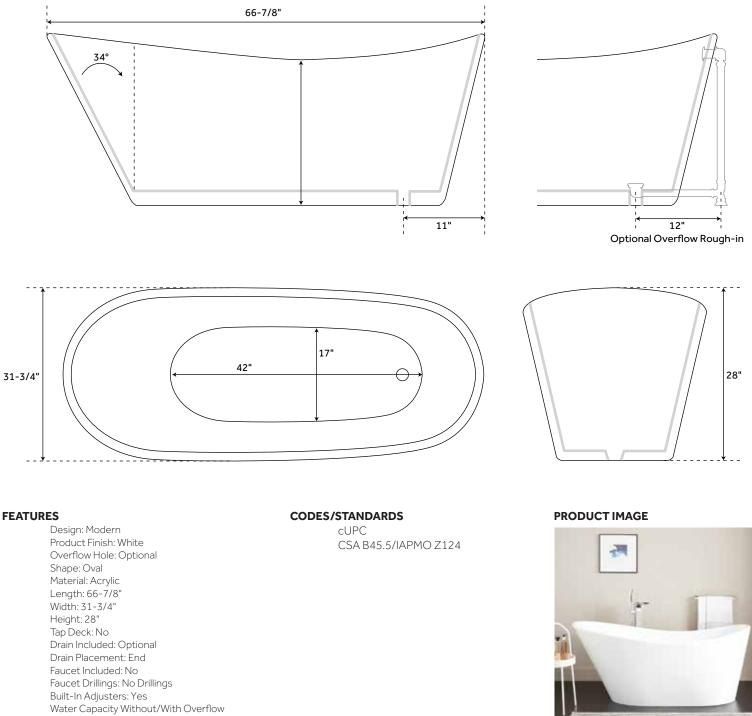
(Gallons): 55/43 Water Depth Without/With Overflow: 18"/14" Tub Weight Uncrated (lbs): 105
