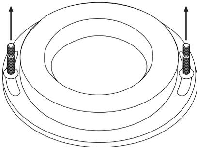
3. When the wax ring and bolts are attached, lift the toilet and align the mounting holes with the anchor bolts on the floor for proper placement.
