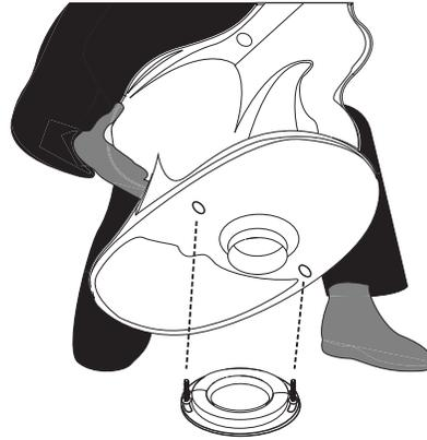
4. Set the toilet down on the floor and press in place to form a tight seal with the wax ring. Do not move the toilet after placement, this could break the watertight seal and cause leakage.
