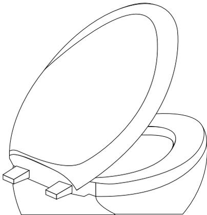
11. If you purchased a bidet seat, connect the three-way valve and hose to the inlet of the toilet seat. Then, using a second hose, connect the opposite end of the three-way valve to the toilet's main shutoff valve on the wall, as shown.
