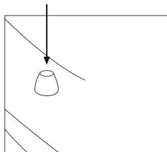
8. If you are installing a two piece toilet, slide the tank bolts through the mounting holes on the top of the base of the toilet. If your toilet has only one piece, move on to step 9.
