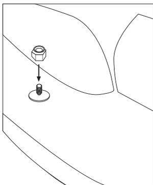
6. When toilet is properly aligned, finish tightening the washers and nuts onto the anchor bolts with your adjustable wrench. Do this gradually, alternating from one bolt to the other until both are tight. Be sure not to overtighten as this could cause cracks and damage the base of your toilet.
