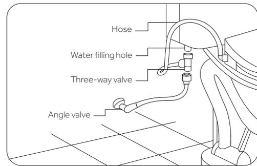
12. If you did not purchase a bidet seat, connect the water supply tubes at the bottom of the tank. Turn on the water supply and flush the toilet several times to check for any leaks around the back or base.
