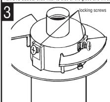
POSITION THE FITTER over the post as shown. Tighten the locking screws. Install light bulb into socket. Be sure to use bulb with wattage no greater than specified for this fixture.
