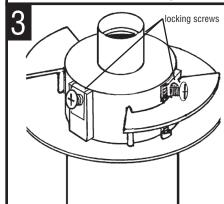
POSITION THE FITTER over the post as shown. Tighten the ATTACH GLOBE TO FITTER. Slide edge of globe between filler locking screws. Install light bulb into socket. Be sure to use and one flange. Push other flange into globe. Center globe bulb with wattage no greater than specified for this fixture.
