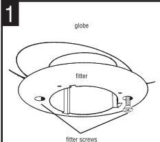
REMOVE GLOBE: slide fitter to side of the globe and lift out.
