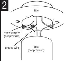
ATTACH BLACK FITTER WIRE to the black supply wire, white fitter wire to the white supply. Use wire connectors (not provided). Connect bare fitter ground wire to the ground wire from the power supply.
