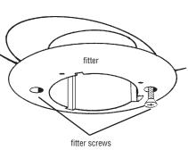
REMOVE GLOBE: slide fitter to side of the globe and lift out
