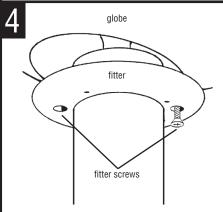
ATTACH GLOBE TO FITTER. Slide edge of globe between filler and one flange. Push other flange into globe. Center globe on fitter. Tighten two fitter screws to secure globe to fitter.
