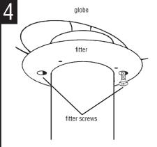
on fitter. Tighten two fitter screws to secure globe to fitter.
