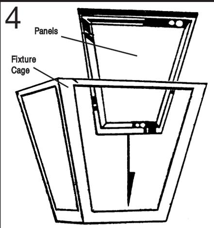
INSTALL PLASTIC PANELS, textured or beveled side out, by sliding panels down cage in slots on inside of cage. Make sure panels are all the way down into seats in cage
