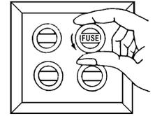
Screw-in type fuses - unscrew the fuse or fuses that control the power to the fixture or room you are working in.
