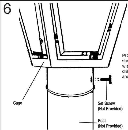
POSITION THE FIXTURE over the post as shown. For permanent mounting, fasten with set screw at hole in post collar by drilling hole at same location through post and securing with screw.
