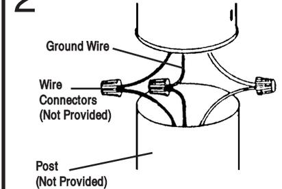
CONNECT THE WIRES. NOTE: Attach black fixture wire to black supply wire, white fixture wire to white supply wire. Do not mix them up. Use approved electrical tape or wire connectors (not provided). Connect bare fixture ground wire to ground wire from outlet box. NEVER CONNECT GROUND WIRE TO BLACK OR WHITE POWER SUPPLY WIRES.
