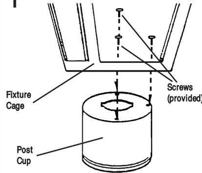
FASTEN THE CAGE to the post cup with the 3 screws provided.
